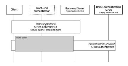
Fig. 1. Customary construction of a tunnelled authentication protocol
