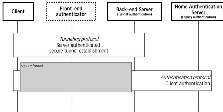
**Fig. 1.** Customary construction of a tunnelled authentication protocol
